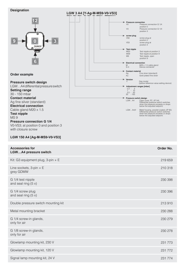
Differential pressure switches for air, flue and exhaust gases Pressure switch for gas
